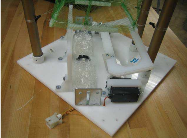
Football grasping system with the server and ball reception sensor
