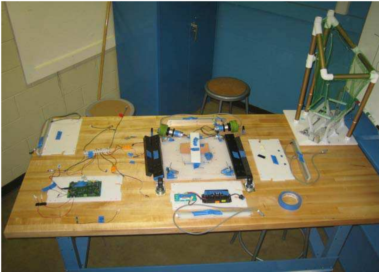
Completely disassembled receiver with the electronic system on the left, structural components in the middle, and receiving arm on the right
