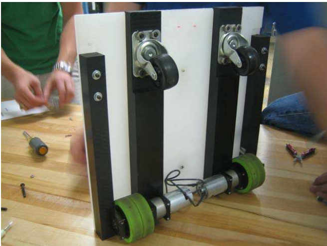
Bottom drive system before removal. The wheel and motor anchors doubled as effective support systems
