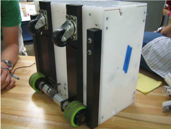
Receiver's bottom drive system with the powered green wheels and free spinning plastic wheels on top
