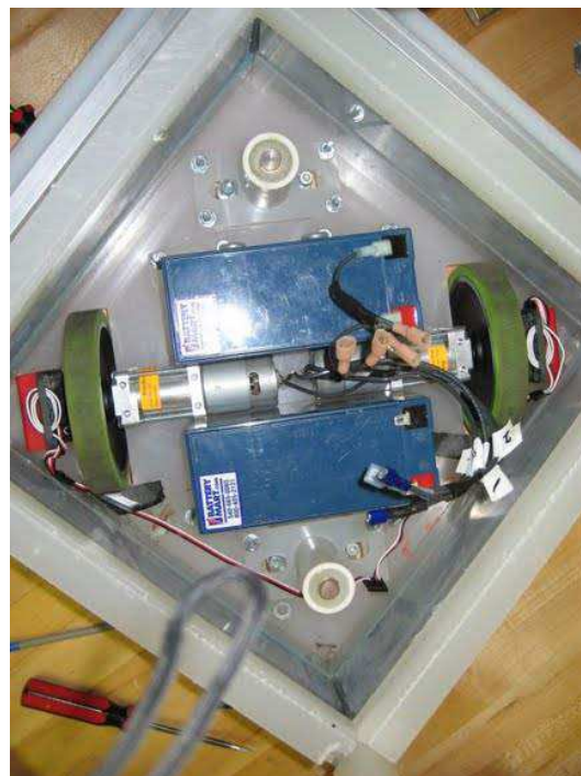
The drive system for the robot including wheels, gearboxes, motors, battery packs, and shock absorbers.
