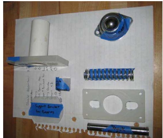
The components of the shock absorber assembly. From left to right are the spring guide, support bracket, spacer, ball bearing and housing, spring, mounting bracket, and shock shaft.
