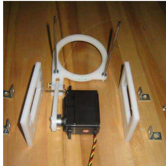
Exploded view of the ball-loading assembly including the motor, supports, and loading arms.
