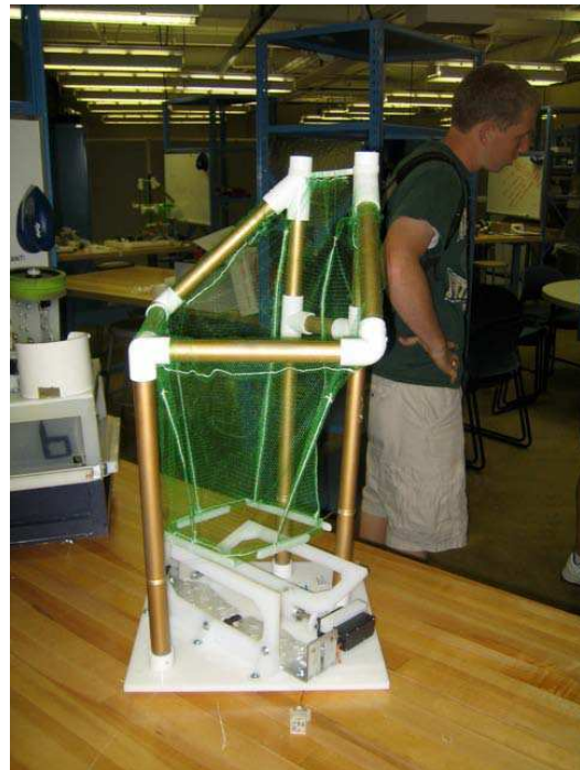
Receiver's top netting and ball grasp pre-assembly
