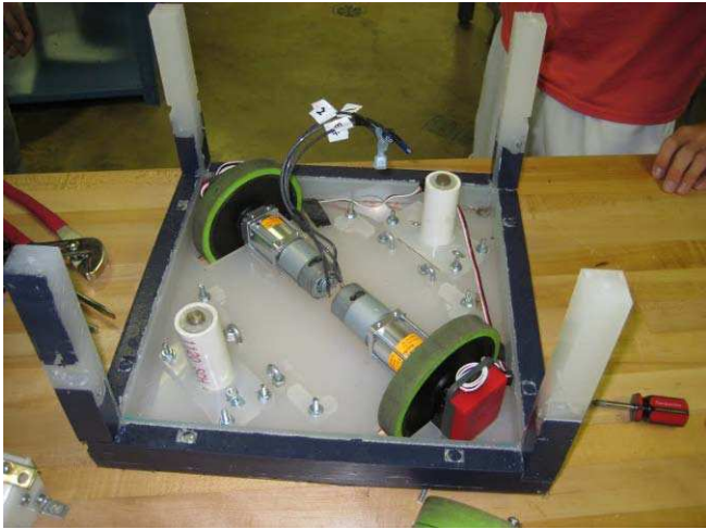
Base Assembly with the side plates and electrical assembly removed.
