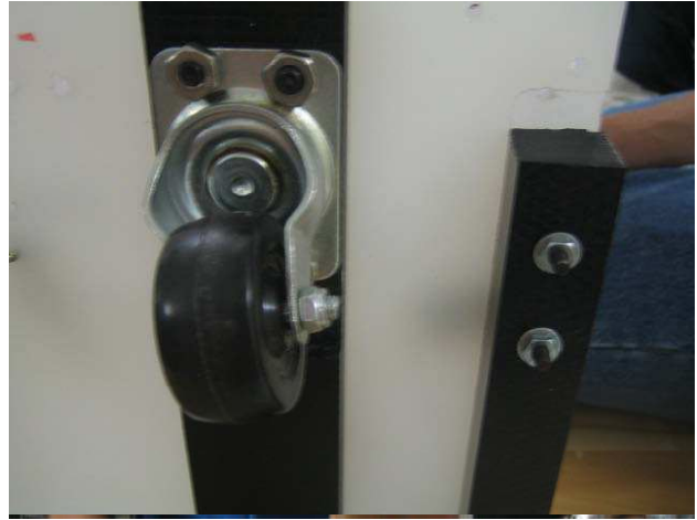
Free coasting wheel in both front corners of the receiver
