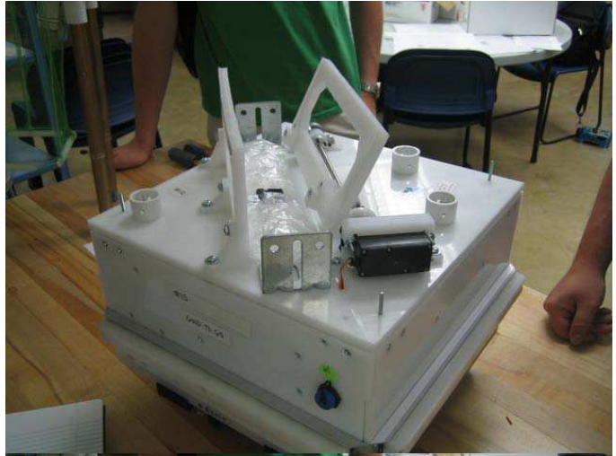
Receiver with top netting and support removed, shows clamping arms
