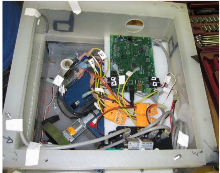
Robot with top top mounting plate removed. From top to bottom the components shown are the processing board, batteries, wheel motor, and tackle sensor.
