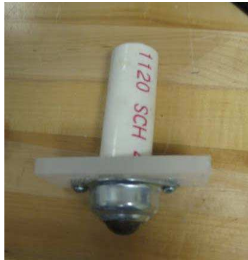
Shock absorber ball bearing, housing, and spring guide.
