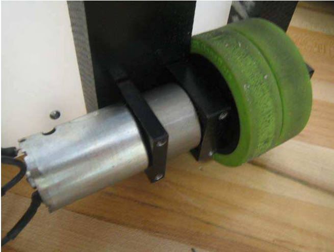
Receiver's driven wheels and motor, one in each back corner
