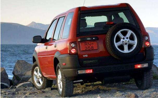
There are two downsides of having the spare in this position: the first is that it obscures rear vision. The second is that it's extremely vulnerable to damage when reversing. If you back into a lamppost, the spare tyre will quite likely distort the whole rear door. This won't be cheap to repair.
