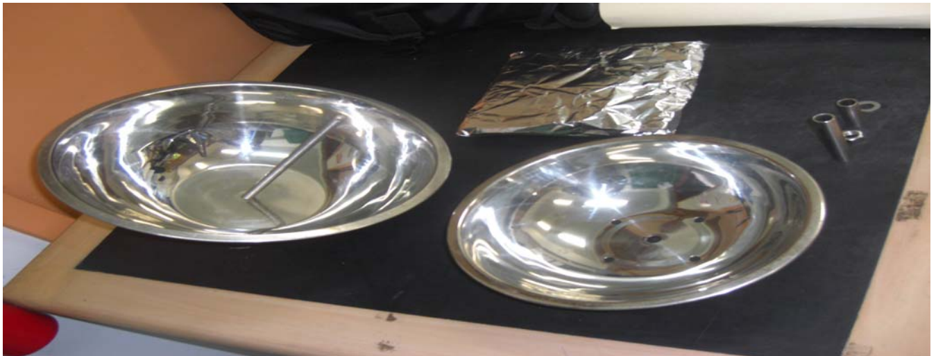
3a. Stainless steel bowls with diameters of 30 cm and 24 cm.
