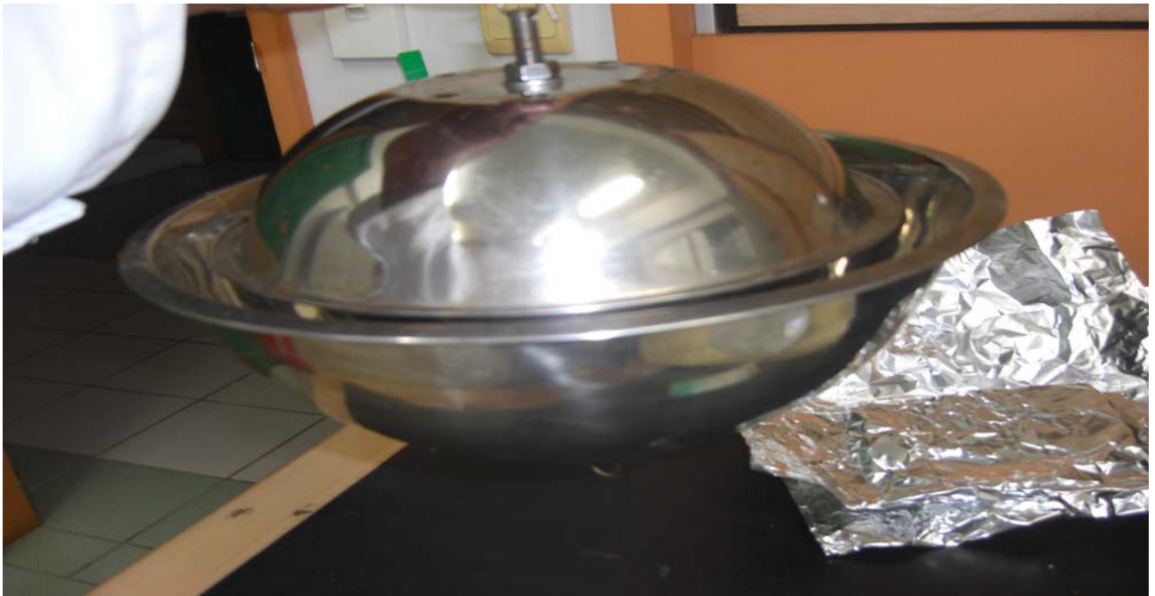
3h. The PAS sampler is ready for deployment onto monitoring site.
