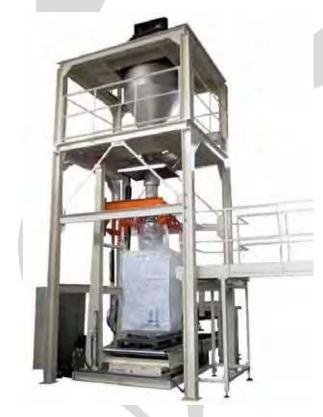
From the feeding hopper the product falls into the weighing hopper through a feeder controlled by the control unit. The weighing done is discharged thought the butterfly valve, which is located on the bottom of the hopper, into the bag, which was previously positioned by the operator in the filling area (the suspenders are hooked to the hooks and the bag mouth to the feeding mouth). The inflation device of the bag allows the complete extension of the bag before the filling phase.
