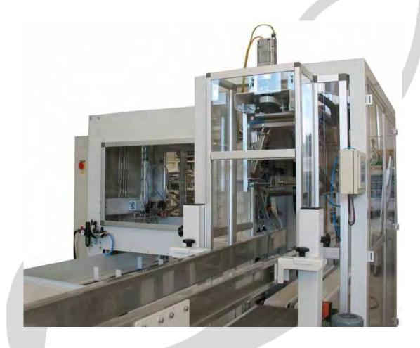
The **BL-OM** bagging machine is a compact fully automatic packaging system. Its design allows the bagging of powders and granules into pre-formed open-mouth bags. The machine is specially studied to facilitate an easy cleaning. The bag spout is featured to allow its simple and quick change with regard to the different bag sizes.
