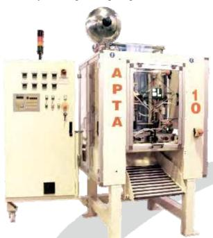
The Apta 10 is a FFS bagging machine, which uses a PE alimentary tubular film from a reel. The film is unreeled by two rubber chains. The unwinding is controlled by encoder to determine the length of the bag. Before such chain unit, a blade opens one side of the tubular film to
