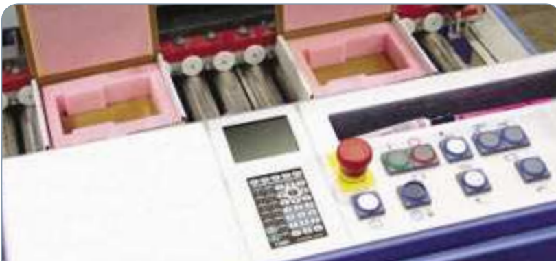
The components of the QTERM-G55 (module) were integrated into the panel of this packaging machine.
