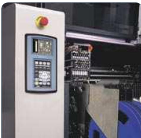
A pick and place machine is controlled by a panel-mount QTERM-G55
