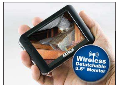
Detachable wireless 3.5" color TFT LCD display
