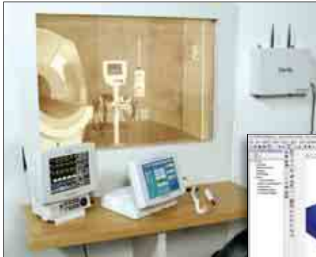
(Above) Figure 3a: An MRI contrast-injection system consisting of a remote control panel that interfaces to the injection head located in the treatment room through a wireless link. A new phototransducer experienced electromagnetic interference and required shielding that was optimized using COMSOL Multiphysics.
