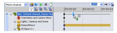
**Note:** The zoom keys • allow you to zoom in and out on the time line. Right-clicking on the timeline key allows you to manually input the desired simulation time.
