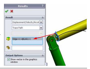
**Note:** The resulting trace path is by default shown with respect to the fixed ground. To show the trace path with respect to another moving component, one would have to select this reference component as a second item in the same selection field.
