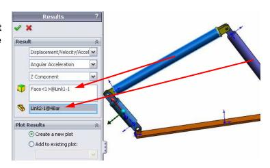
**Note:** The triad on the Link2 component indicates the output local coordinate system. Contrary to the global coordinate system which is fixed, local coordinate systems may rotate.. In our case, the selected local coordinate system will rotate because Link2 component rotates as the mechanism moves.
