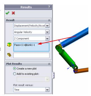
The plot shows the variation of the angular velocity of the center of mass for Link1 as function of time.
