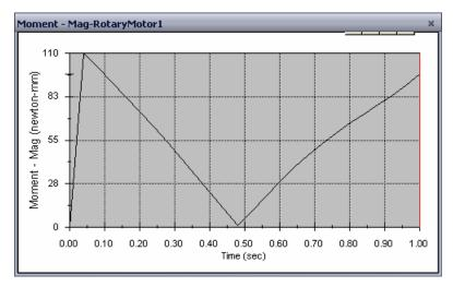
The required torque is about 110 N-mm
