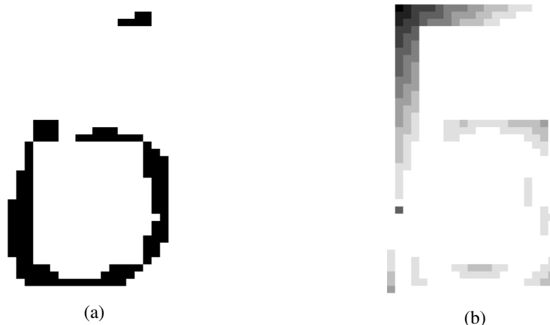
Figure 5 - The final stages of the template match. (a) Pixels that overlap between the template and the image. (b) Distance map between template and image. Darker pixels are farther away.
