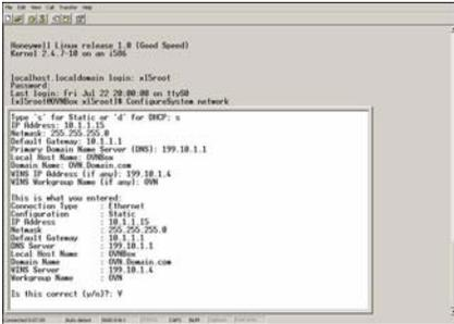
Fig. 20. Configuring Static IP Address.
