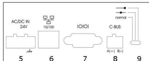
Fig. 6. Excel 5000™ Open View Net Rear Panel.
