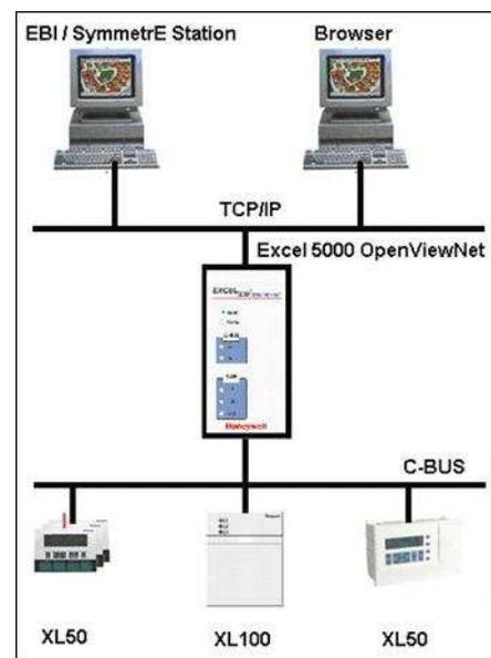
Fig. 1. Excel 5000™ Open View Net Architecture.
