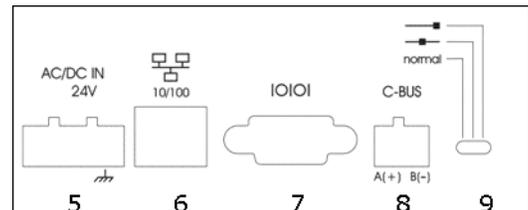
Fig. 5. Excel 5000™ Open View Net Rear Panel.
