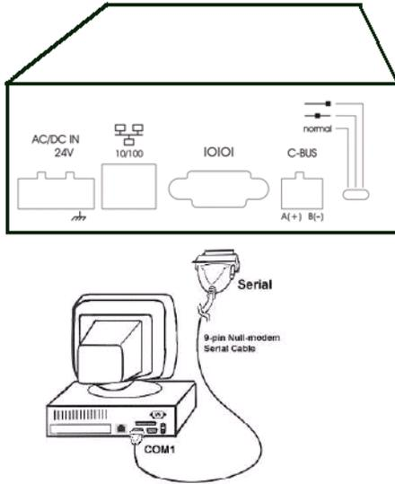
**Fig. 7. Connecting PC to Excel 5000™ Open View Net's Serial Port.**
