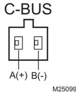
Fig. 2. Field bus connection.
