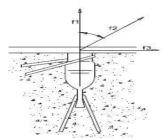
A lateral reinforcement bar is required for lifting angles in excess of 15°. The bar should be fitted in close contact with the socket in the opposite direction of the angle of the lifting force
