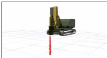
2. The injection of cement mortar creates root piles that increase the structural safety of the foundation
