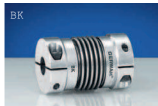
Metal bellow coupling with clamping hubs; 0,2-300 Nm Technical data page 10
