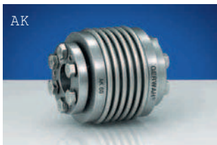
Metal bellow coupling with inner conical hub; 30-5000 Nm Technical data page 8
