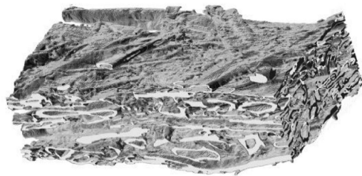
Tomographic image of a paper fiber web
