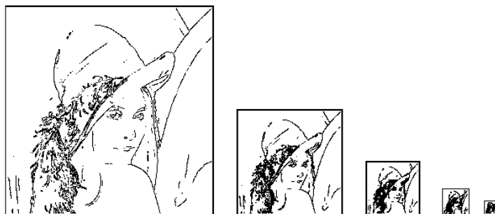
The selection masks at several scales. Since they are binary, an AND-operation is all it takes to mask out the desired coefficients. The masks are independent of each other. Sharp edges are present at all scales, but other features are only present in some. This can be exploited in texture separation.
