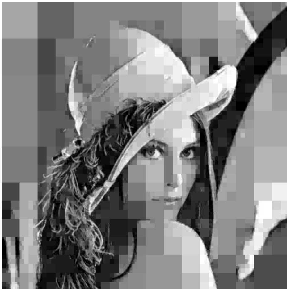
The image of Lenna coded and reconstructed using wavelet coefficients selected by a binary edge map. The Haar filter is used, which introduces false edges on the larger scales.
