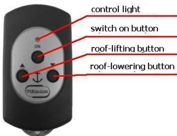
Picture 26: Remote control for the lifting and lowering of the roof
