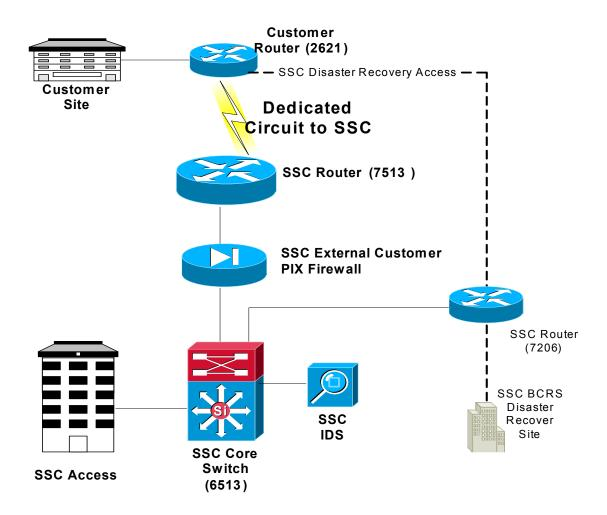
Figure 1. — High Level Diagram of [CUSTOMER AGENCY]/[SHARED SERVICE CENTER] Connectivity
