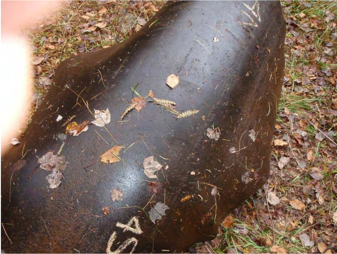
Figure 9: Piece 4 exhibiting corrosion
