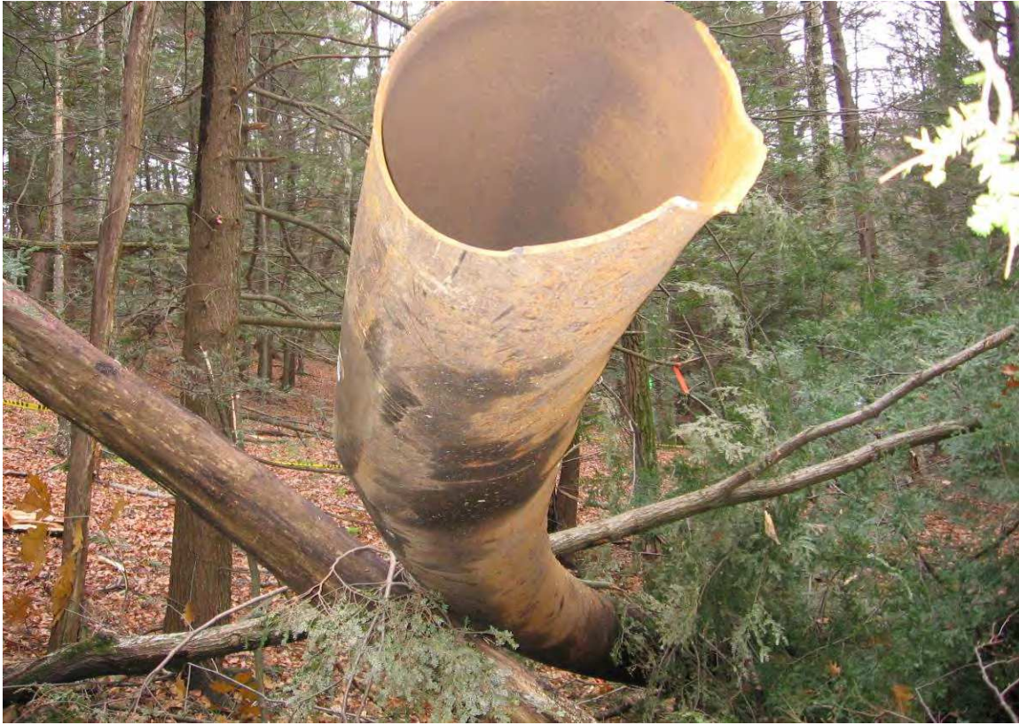
Figure 7: Bent 21.7 foot section of pipe in swamp
