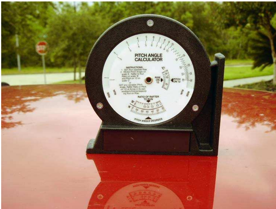
Figure 6: Typical roof slope meter used for measuring roof slope.
