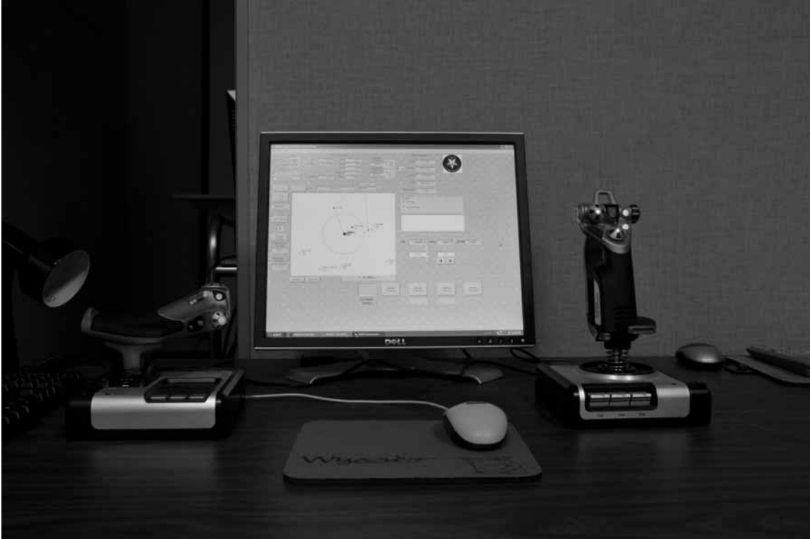
Figure 1. UAS control station simulation used in the experiment.
