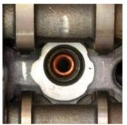
If the shaft is very strongly polluted it is advisable to occasionally clean the shaft, between brushing, with compressed air or a vacuum cleaner. Caution, wear safety goggles! Repeat the operation until the injector shaft is shiny clean.
