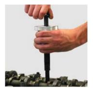
Place the sealing ring extractor p/n PZ471 6039070 in the shaft with the slide hammer p/n PZ 485 903 90750 screwed on and knock, with feeling, the claw into the hole of the sealing ring. Remove the slide hammer.
