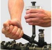
In very severe cases the injector can be removed with the pivot adapter p/n PZ 485 903 8440 and the slide hammer p/n PZ 485 603 90750. Remove the O-ring, slide the pivot adapter p/n PZ 485 903 8440 on the handle and return the O-ring in the groove on the handle. Screw the handle on the diesel connector and the slide hammer on the pivot adapter. Knock by simultaneously rotating and striking the injector from the shaft.
