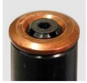
Get a new sealing ring and place it on the extraction claw in order to adjust the grip depth. The length of the claw can be changed by turning. The claw is optimally adjusted when the collar protrudes minimally over the sealing ring. If the collar protrudes too much, the extractor will jam in the bore of the nozzle and can not grip the sealing ring. Also is there a risk of damaging the cylinder head. If the claw is not adjusted enough, then the extractor will not grip the sealing ring.
