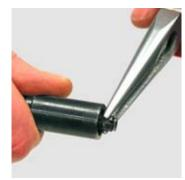
After being used several times it can happen that the four claw elements get overstretched and do not fit in the sealing ring anymore. This can be corrected by squeezing them together with a pair of longnosed pliers.
