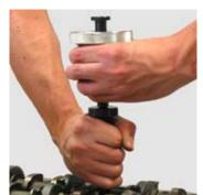
Screw the slide hammer on the sealing ring extractor and knock with feeling the copper seal out of the injector shaft .
