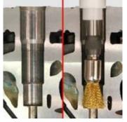
Remove the sealing plugs by means of the setting tool. Guide the brush again in the injector shaft and repeat shortly the cleaning of the sealing seats.
