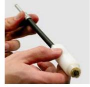
Plug the brass end brush p/n PZ 485 903 9011 onto the flexible shaft. Slide the plastic guide p/n PZ 485 903 9016 on the flexible shaft and end brush.
