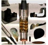
Measure the diameter of the removed injector and select the appropriate brass brush: Ø18; p/n PZ 485 903 9132 Ø19; p/n PZ 485 903 9131
