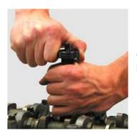
Grip the sealing ring by turning the knurled actuator and holding the knurled pipe.
