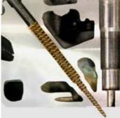
Remove the glow plugs. Clean the glow plug shafts with stepped brass wire brush p/n PZ 485 904 9026.
