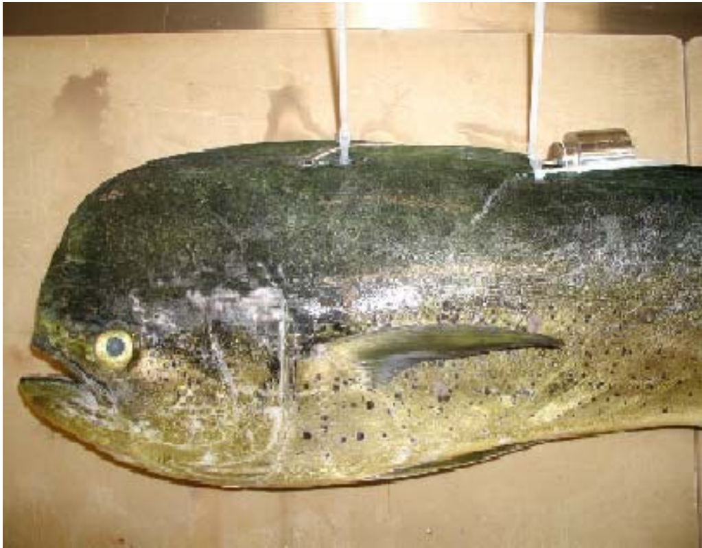
Figure 3: Mahi-mahi with secured temperature probe.
