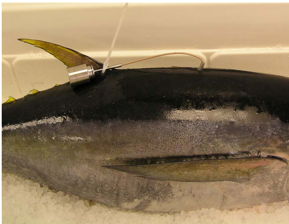
Figure 4: Yellowfin tuna with secured temperature probe.
