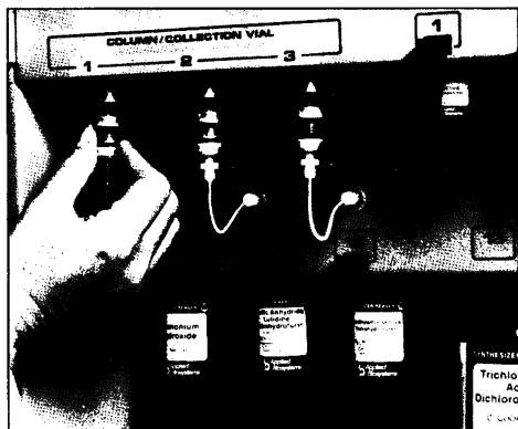
Three synthesis columns can be operated independently and simultaneously, tripling the productivity of the Applied Biosystems Model 380A DNA Synthesizer.
