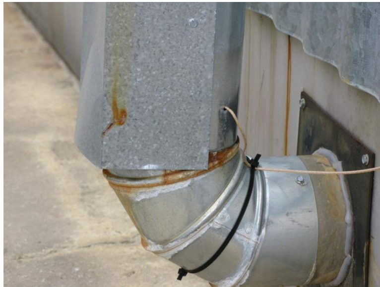
Figure 3-10: Thermocouple in mounted in an exhaust stack
