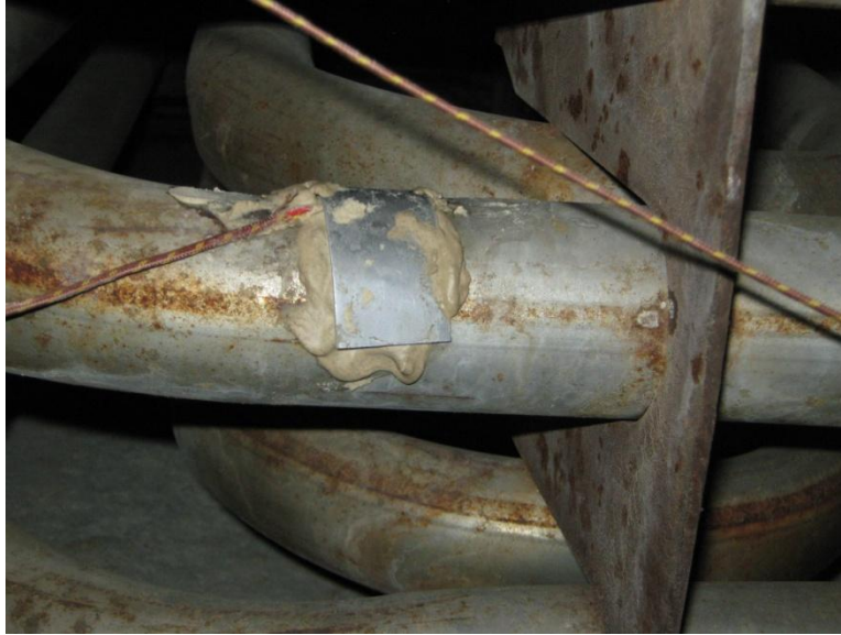
Figure 3-7: Close up of a thermocouple mounted on a Taylor heat exchanger
