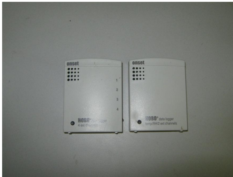
Figure 3-12: HOBO data loggers used to monitor barn temperature and static pressure
