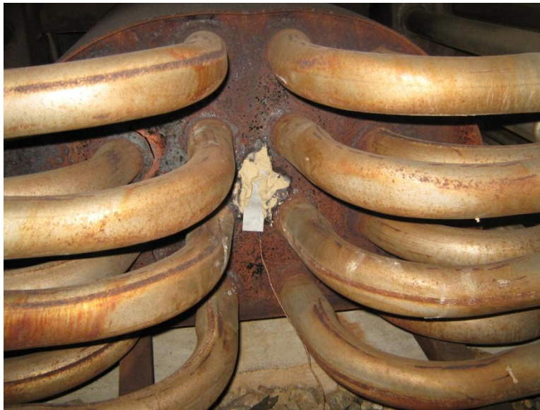
Figure 3-8: Thermocouple mounted on Taylor heat exchanger combustion chamber
