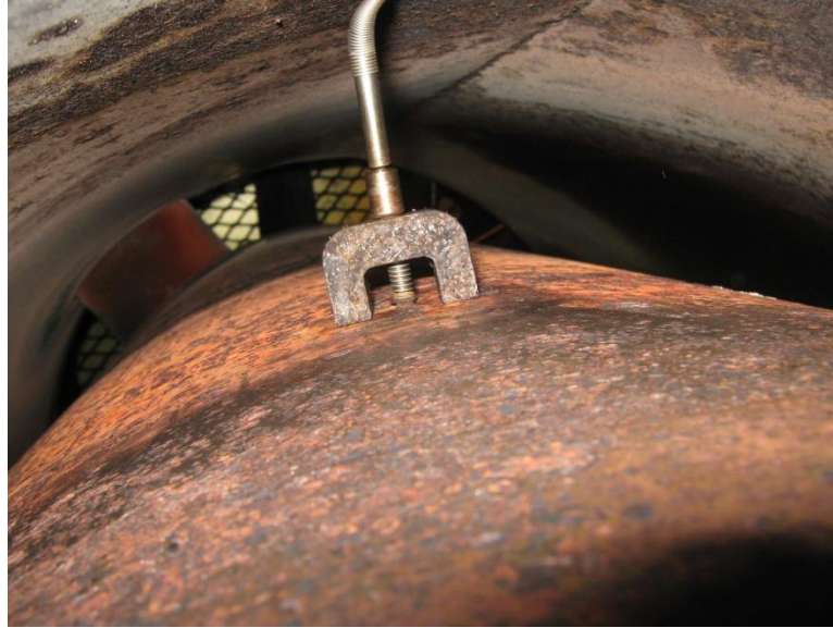
Figure 3-9: Magnetic thermocouple mounted on a Long heat exchanger
