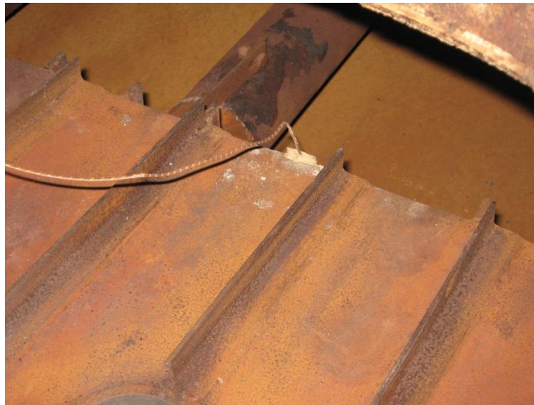
Figure 3-6: Thermocouple mounted on Reddick Manufacturing heat exchanger
