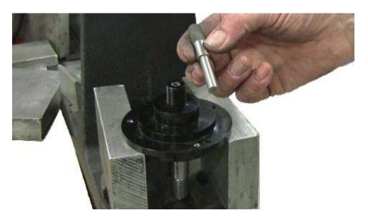
Get a punch of smaller diameter than the shaft and press out the shaft.
