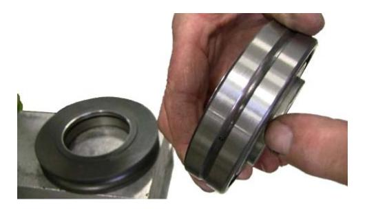
Take the Tension Wheel. 2 snap rings will hold the bearing assembly in place. The front of the wheel is the side with the grease fitting.
