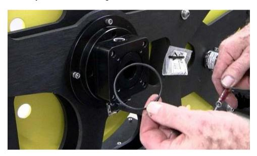
Note the size of the gap between the coupling and the encoder body.
