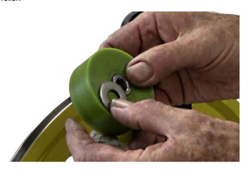
When replacing the pressure wheel, you must compress the tensioner to allow the bolt to go into the wheel – tighten the bolt.
