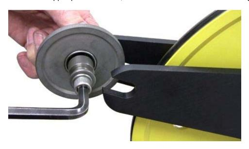
Loosen the lower pressure roller, move it to the end of its slot and retighten the bolt
