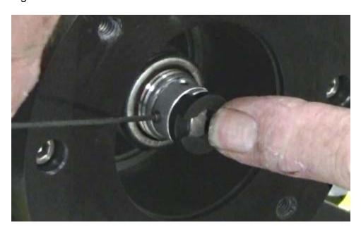
Lubricate and replace the O ring on the adapter – DC111 lubricant works well in this application.
