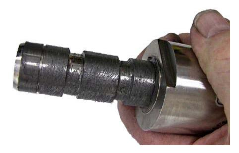
The flat side of the load pin will flange up to the guide plate on the frame.
