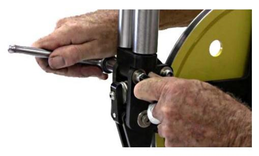
When replacing the keeper roller, make sure you have a flat washer on each side of the roller.
