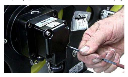
Place the Allen wrench in a set screw hole and exerting force, lever the encoder stack away from you towards the measuring wheel, snug up the set screw.
