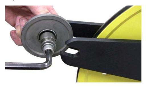
Pull the wheel up and out of the frame.
