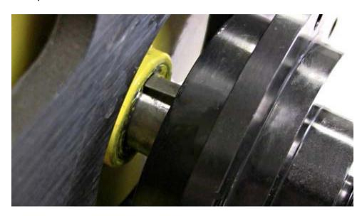
Rotate the hub so that the grease fitting faces to the right and the 4 screw holes on the hub align with the holes on the frame.
