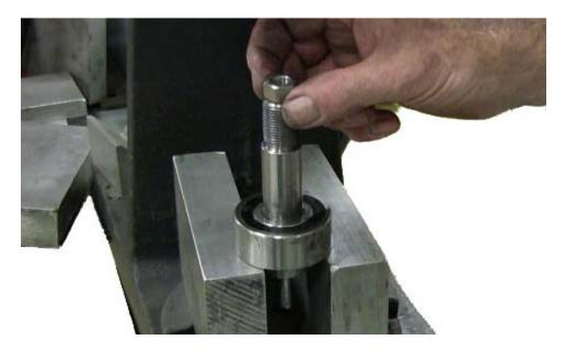
Place the new bearing on the shaft and snug as much as possible manually.
