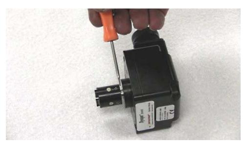
With the small Allen wrench, loosen the 2 set screws that hold the coupling on the shaft of the encoder.
