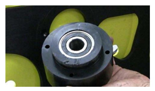
Remove the retainer clip that holds the bearing in place in the hub. It can normally be removed and replaced with no special equipment. Install the new bearing and the retainer clip.
