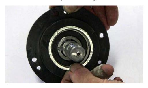
You now need to press the shaft and the bearing out of the hub. You will usually need a press to both remove and reinstall the bearing and shaft. Set up your press to allow pressing the shaft and bearing out through the bottom of the hub.
