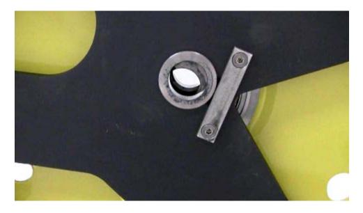
Note that the load pin has a flat notch on one side.
