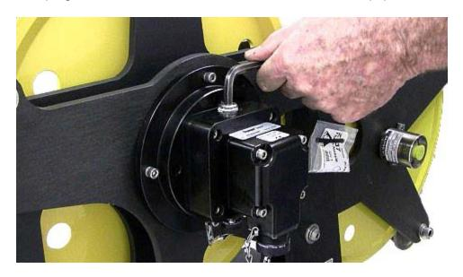
Next remove the 4 encoder screws. Hold the encoder as the last screw is removed or it will fall from the adapter body.
