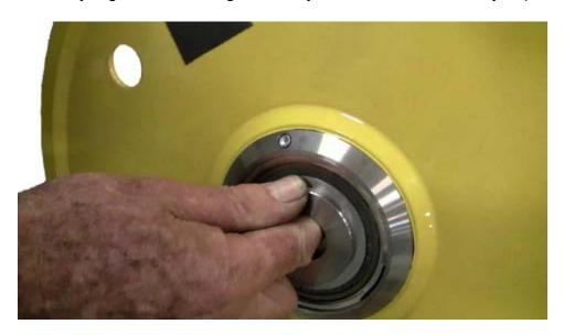
**Lubrication** – use waterproof marine grease and a straight necked grease gun. Use the grease nozzle that comes with the measuring head (in the small plastic bag zip-tied to the frame).
