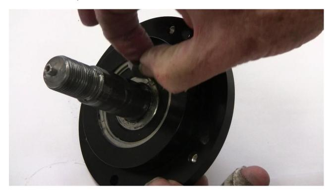
Now remove the retainer clip for this bearing.
