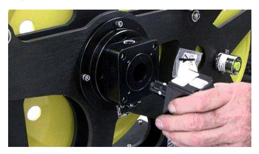
If the plastic coupling is attached to the coupling stack, remove it.
