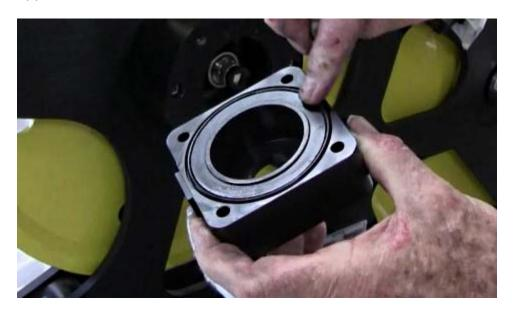
Replace the adapter and all 4 screws – tighten the screws firmly.
