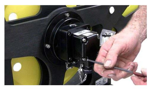
Carefully pull the encoder straight out avoiding contact between the couplings and the adapter.
