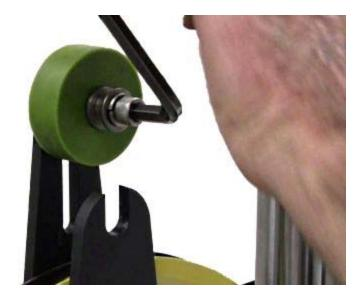
Loosen the upper pressure roller, move it to the end of its slot and retighten the bolt.
