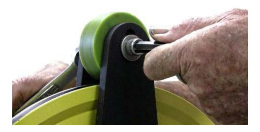
Note that the keeper roller has a flat washer one on each side of the roller that will be used again when the wheel is replaced.
