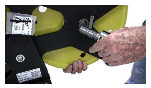
With the load pin removed gently let the tension wheel rest in the frame.
