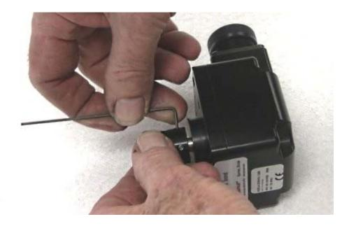
Remove the coupling stack from the shaft.
