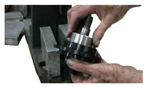
You will now press the bearing with the shaft in it, into the hub.
