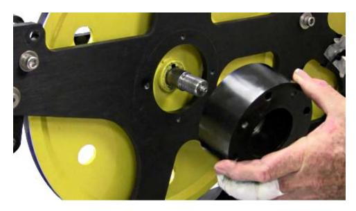
Reinstall and tighten the 4 screws on the hub.
