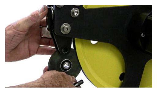
Remove the keeper roller on top of the measuring wheel.
