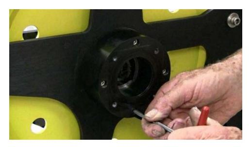
The other half of the hub assembly is on the other side of the frame. Take the dowel out of the wheel.
