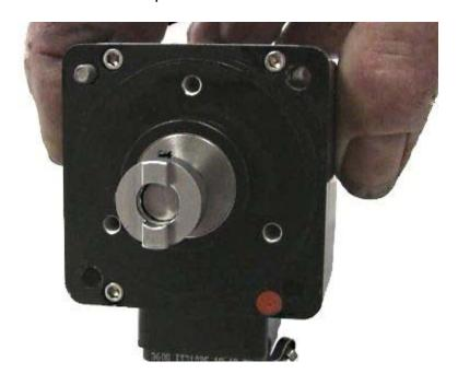
Replace the encoder while looking through the plug hole on the top and rotating the measuring wheel as necessary to get the 2 parts of the coupling to mesh.
