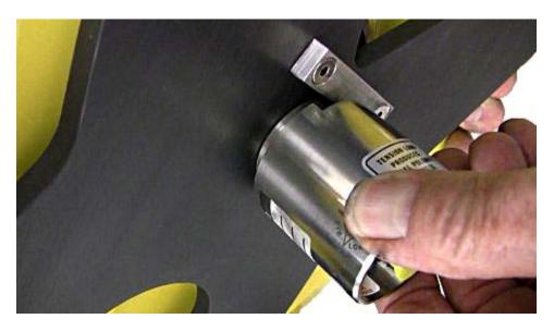
The bearing in the tension wheel has a slot for an anti rotation screw.
