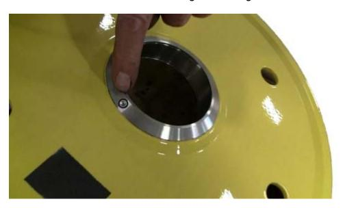
On the BACK of the wheel, install the 1st snap ring.
