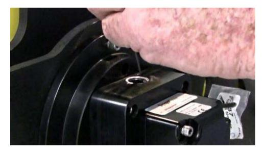
Remove the temporary screws remembering to hold on to the encoder. Carefully remove the encoder taking care to not jar the encoder stack.
