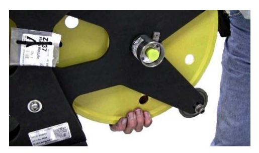
Gently remove the load pin from the wheel hub. The load pin shaft holds the tension wheel in place.
