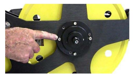
Hold the measuring wheel and remove the hub and shaft assembly – you will probable have to tap on the shaft from the encoder side to get it to come out.
