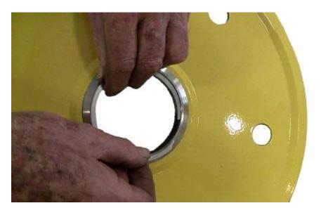
Then turn the wheel over. You should be able to simply insert the bearing assembly into the center hub. \*\*NOTE make sure the small grease hole on the outside of the bearing assembly is placed directly in front of the grease fitting of the bearing or it will not be properly lubricated and the bearing will fail.
