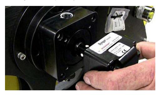
Using a flashlight look in the hole to verify that the plastic coupling has engaged the tang on the measuring wheel.
