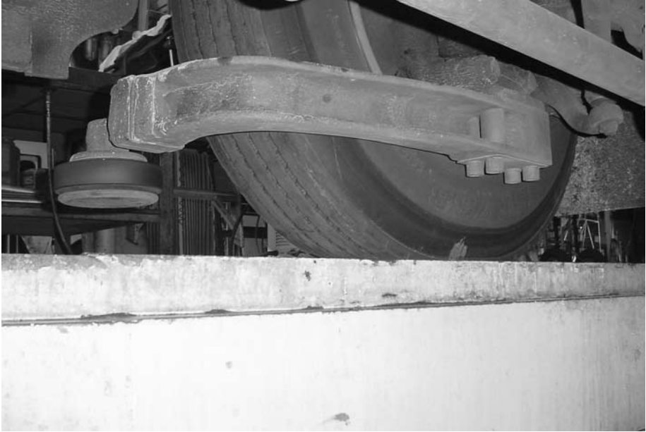
Figure 5. Typical guidearm/guidewheel installation— Mercedes bus in Adelaide
