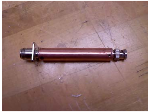
Figure 17: Receiver Structure. BNC Connector and 50 Ohm Load Matching BNC
