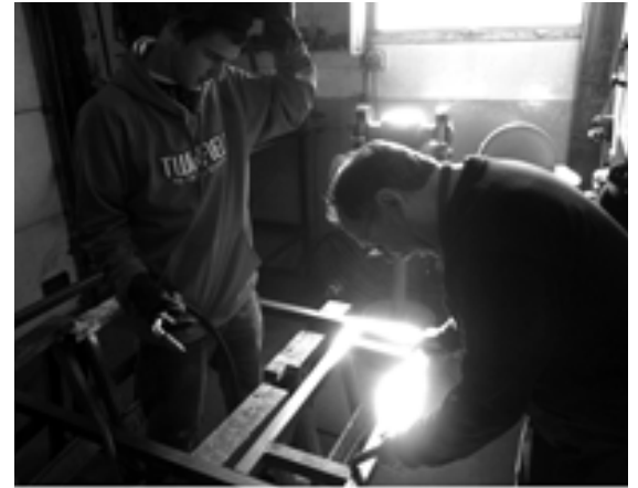
Mark is showing Ryan where to tack the metal, before welding it to the frame
