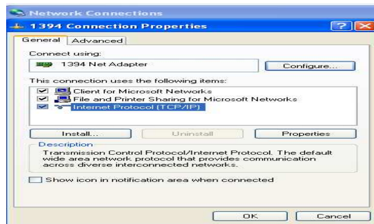
Figure 4.4: Network Connection Setting for Windows based PC
