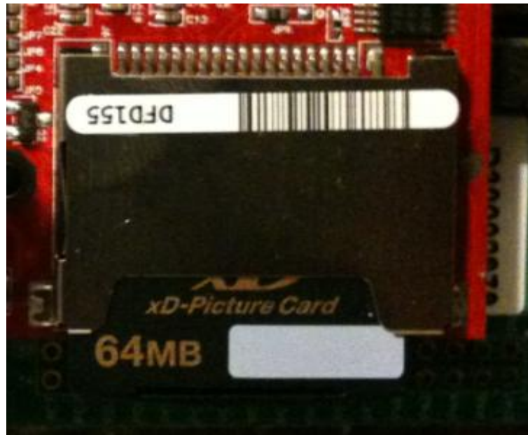
Figure 2.3: Insertion and Removal of xD-Picture Card (64MB)
