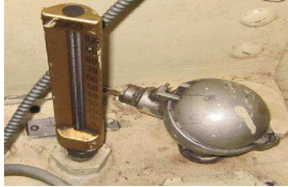
Figure 4.10: Thermocouple for measure shaft temperature.
