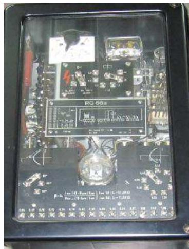
Figure 4.3: Under frequency relay.
