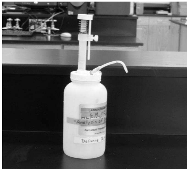
Figure 1. An autopipet. The autopipets should have been calibrated before the start of lab, so please don't readjust them. If you don't believe the correct amount is being delivered, let the instructor know.
