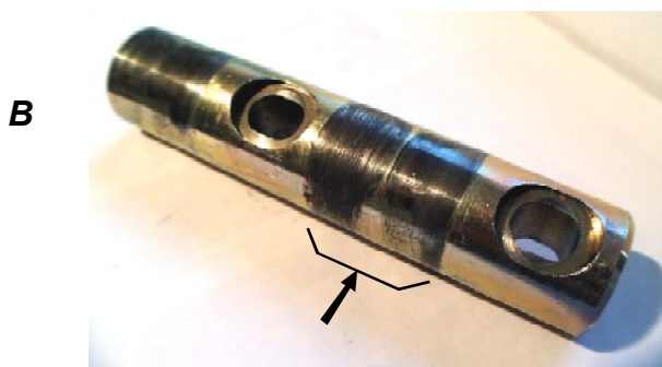
A : Normal condition of the bearing surface. B : Bearing surface damaged, pin to be replaced.
