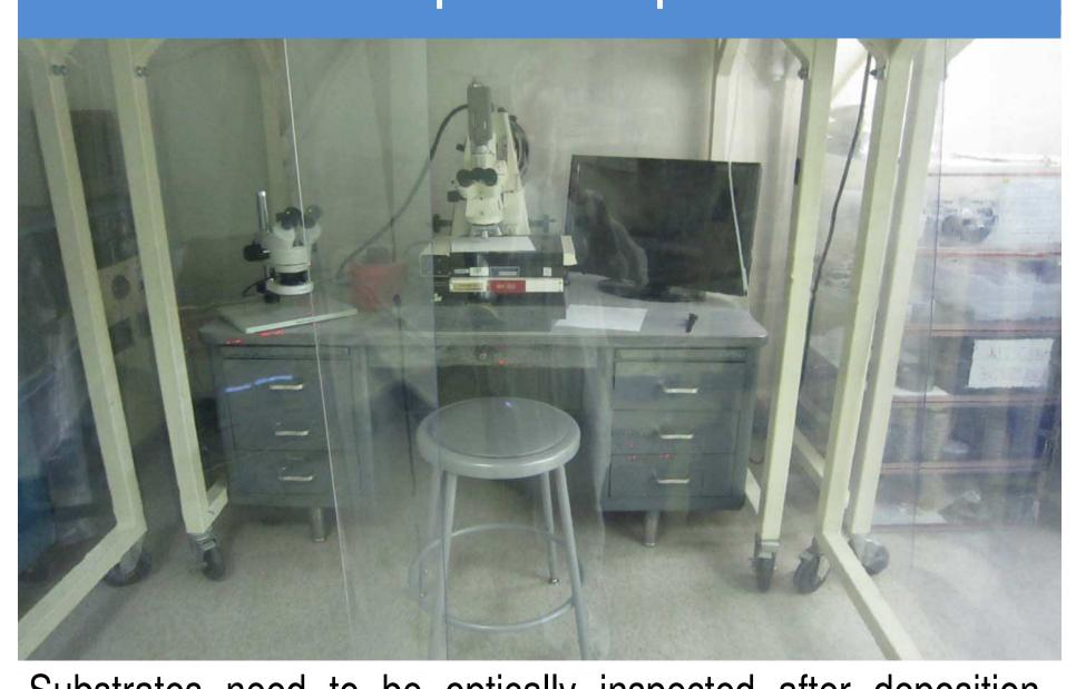
Substrates need to be optically inspected after deposition, photolithography, and etching processes to check against etchdefects.
