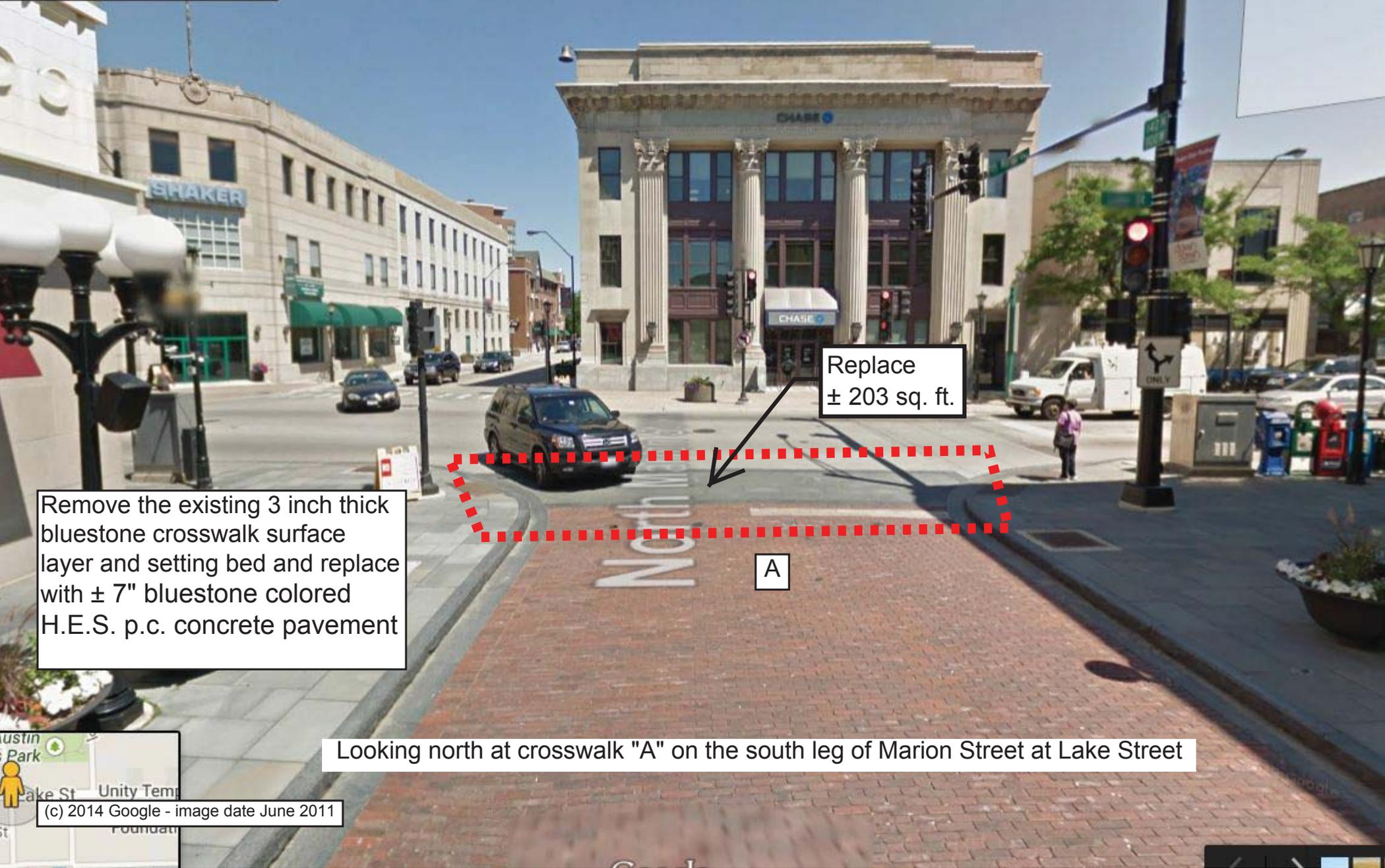
Remove the existing 3 inch thick bluestone crosswalk surface layer and setting bed and replace with  $\pm 7$ " bluestone colored H.E.S. p.c. concrete pavement
