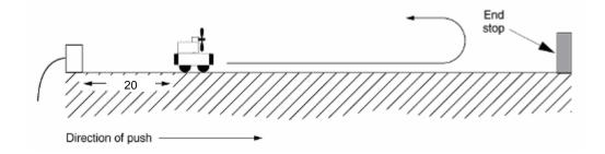
**Prediction 3-5:** Imagine that you start the fan and give the cart a push *away* from the motion detector. It moves away, slows down, reverses direction, and then moves back toward the detector. For each part of the motion—*away from the detector*, at the turning point, and toward the detector—indicate in the table below whether the velocity and acceleration will be positive, zero, or negative.
