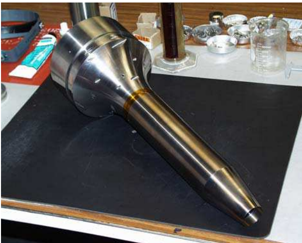
Fig. 2. Penetrator test article. Note the conical nose with tapering bore to prevent bridging during sample acquisition.
