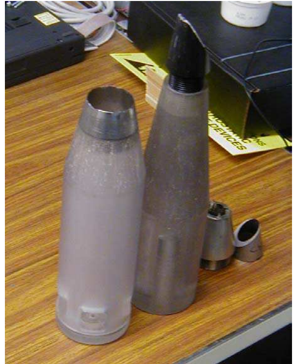
Fig. 3 Small Lexan penetrators used to investigate and optimize nose characteristics for sample coring.
