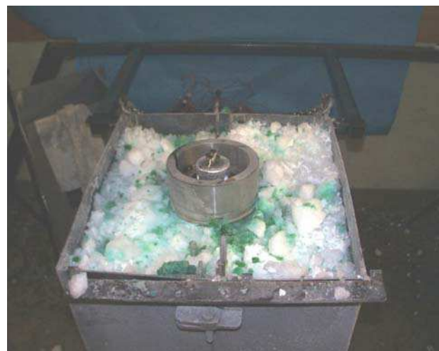
Fig. 9. Penetrator embedded in target. Green ice is due to dye applied to ice at ~3cm depth to investigate stratigraphy preservation. Note the bar at back of penetrator, for actuating sample mechanism.
