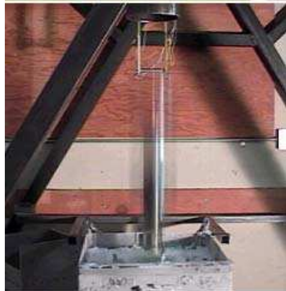
Fig.8 Video frame (using normal camcorder) showing streaked image of penetrator entering target bin. Note the speedometer sensors at top, and the bin location framework.
