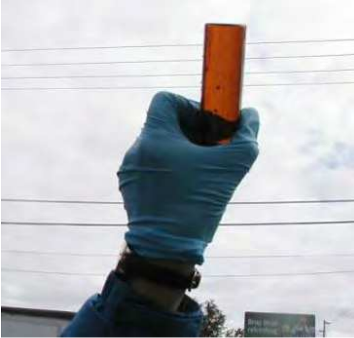
Figure B-6 – Checking a filled VOC bottle for bubbles
