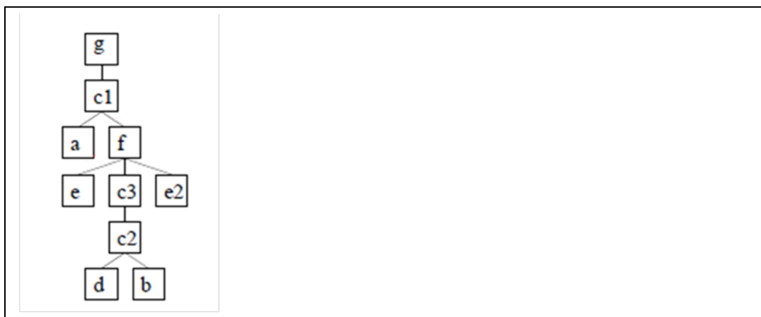
Figure 10. Post-dominator tree for the control flow graph in Figure 9
