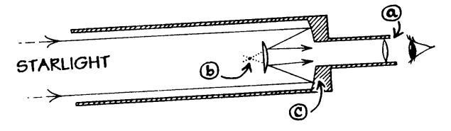
Identify the parts of a Cassegrain **reflecting telescope**: Eyepiece, Primary Mirror, and Prime Focus.
