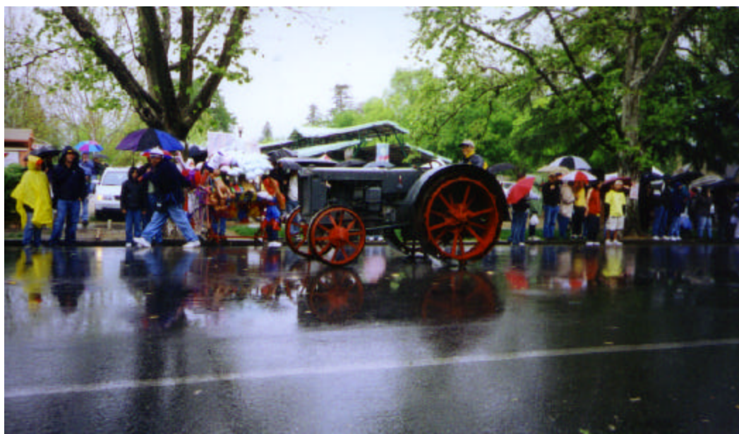
Mikko Solomon driving the Case CO. The steel bands around the rear wheels have flattened out between the wheel “cogs,” giving poor Mikko a bumpy ride and causing the nuts to rattle off the fuel tank strap.
