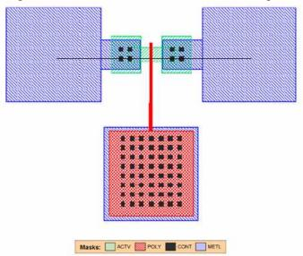
B. Draw top views of the same thin-oxide *MOSFET* (test structure 8) after each of the four photolithography steps. [ACTV, POLY, CONT, METL] (4 Points)
