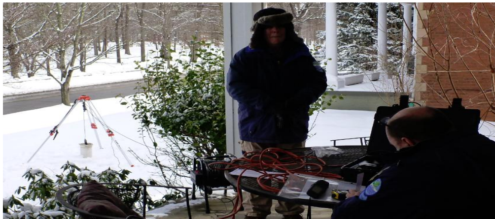
Groundwater staff video logging a water well, Ashland KY. Photograph by DOW staff member Phil O'Dell.
