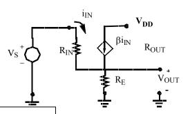
Node equation (KCL) at the output node.
