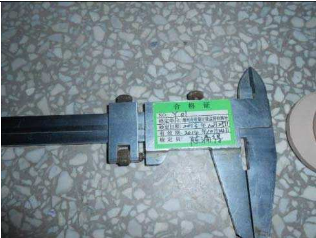
NC 5.7/6.4 The vernier calliper, electric scale were not calibrated timely. Expired date was 24, Oct, 2014.
