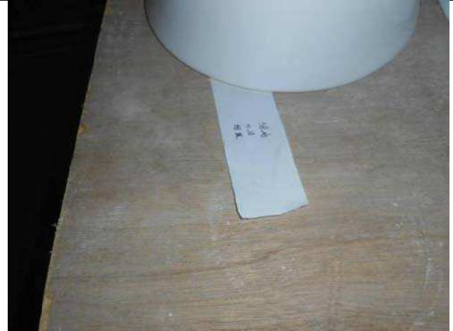
NC 5.5 For WIPs in production workshop, no batch code were used on identification label, deferent batch were not separate storage.
