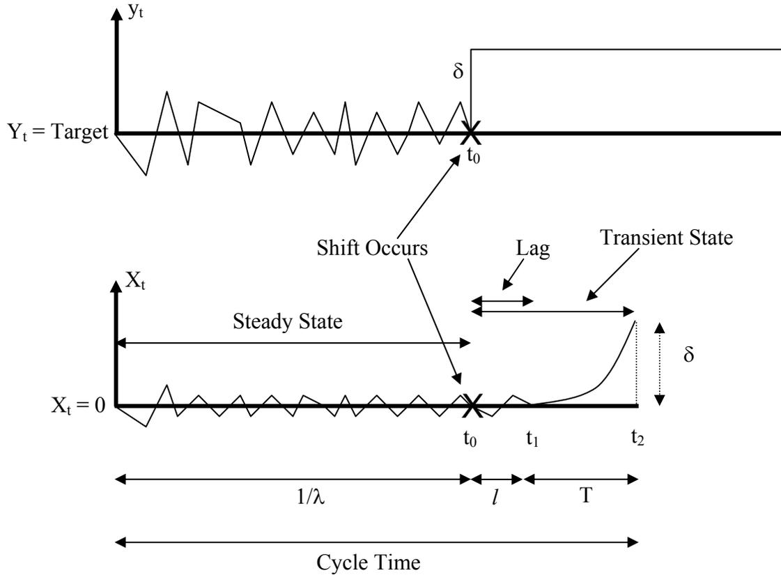
Figure 6.1. Schematics representation of cycle time (APC system).
