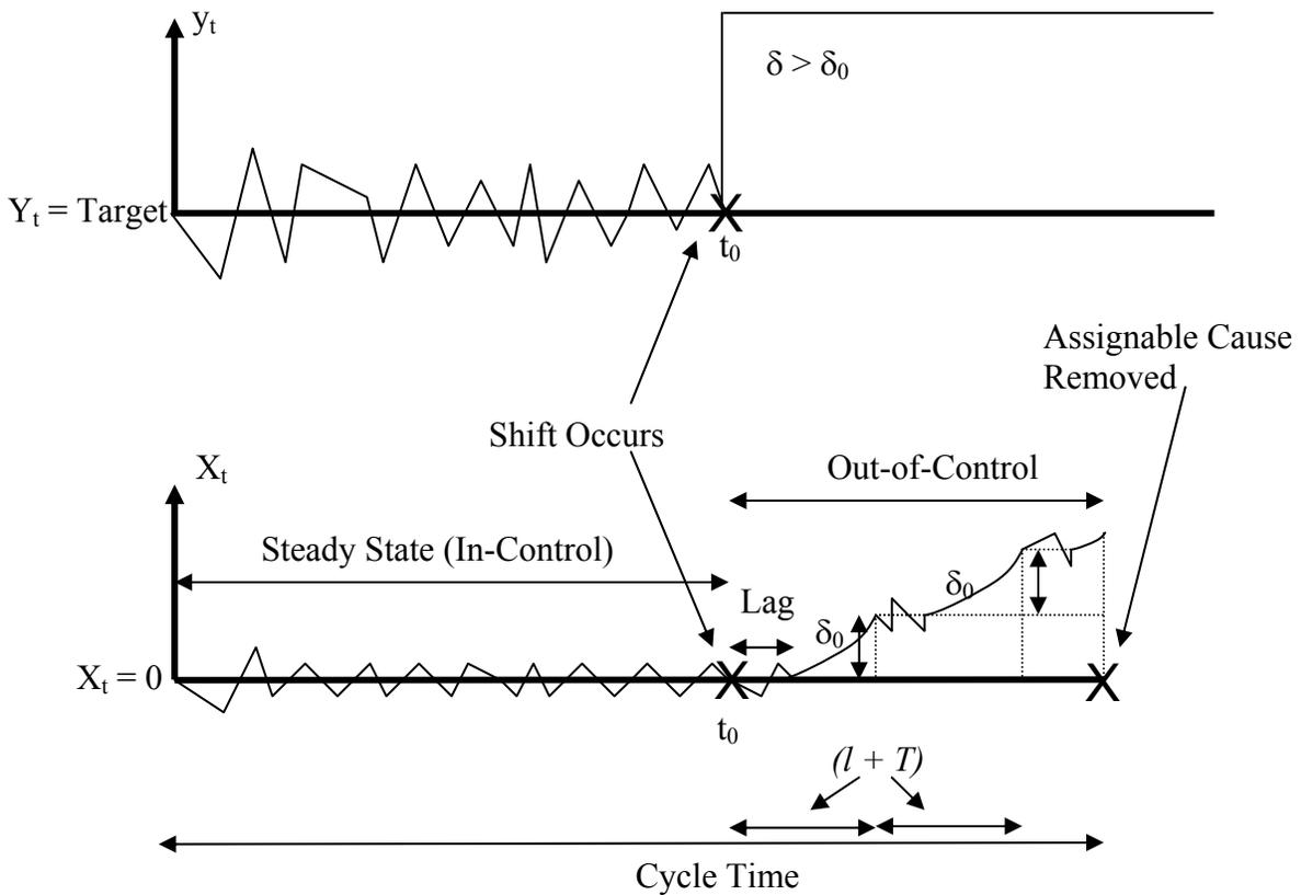
Figure 6.3. Schematic representation of cycle time (ISPC system).
