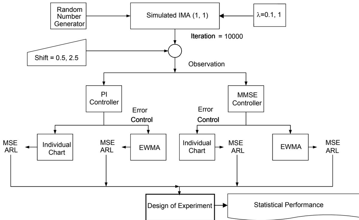
Figure 5.1. Simulation model for statistical performance.
