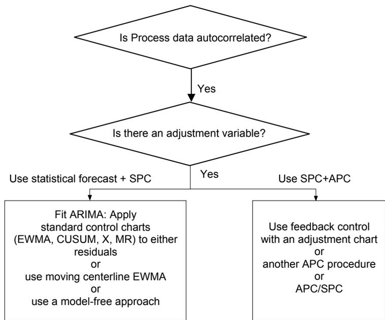
Figure 4.1. Application of SPC to monitor the error and control signals (Montgomery, 2001).
