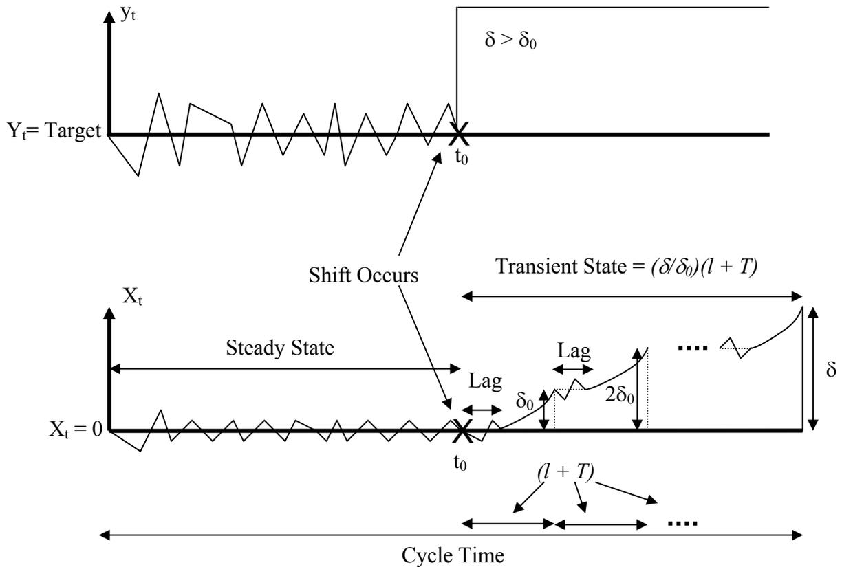
Figure 6.2. Schematic representation of cycle time (APC System,  $\delta > \delta_0$ ).
