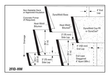
Heat weld a full width piece of one of the cap sheets listed over the installed base felt. Subsequent sheets are to be applied in the same manner, with 4" (102 mm) side laps and 4" (102 mm) end laps over the preceding sheet.
