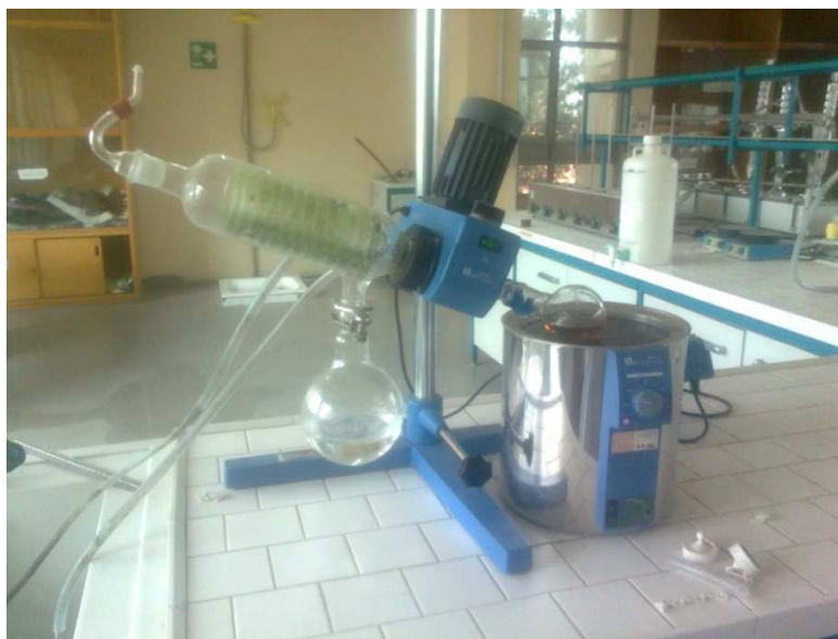
Fig. 3.2: Dichloromethane recovery using Rota vapor from the extracted fleshing oil
