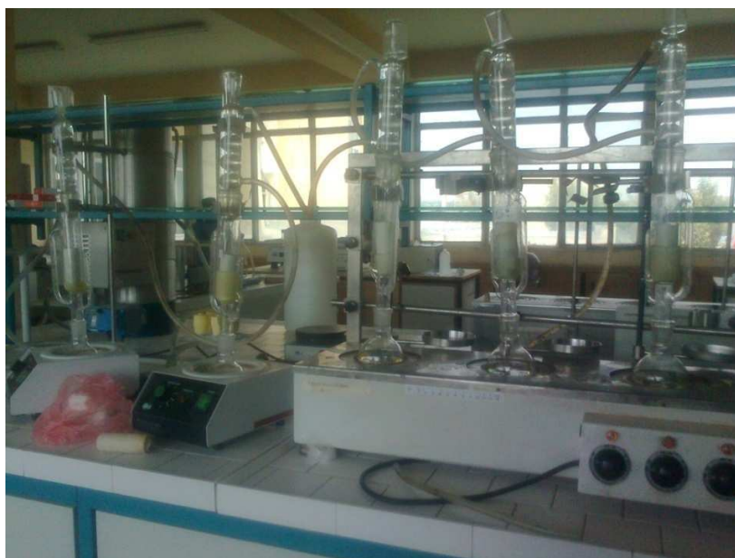
Fig. 3.1 Experimental set-up for Soxhlet Extraction
