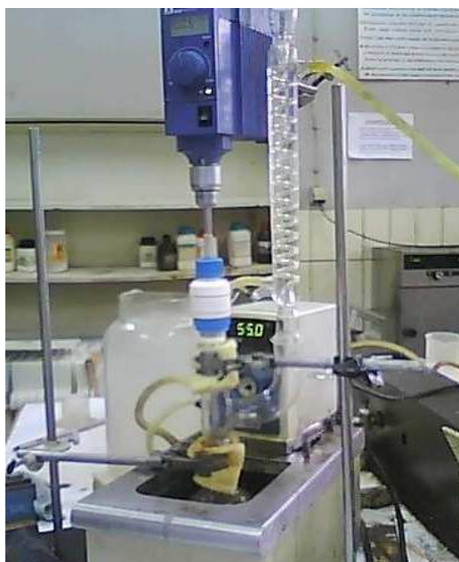
Fig. 3.3: Experimental set up for transesterification reaction
