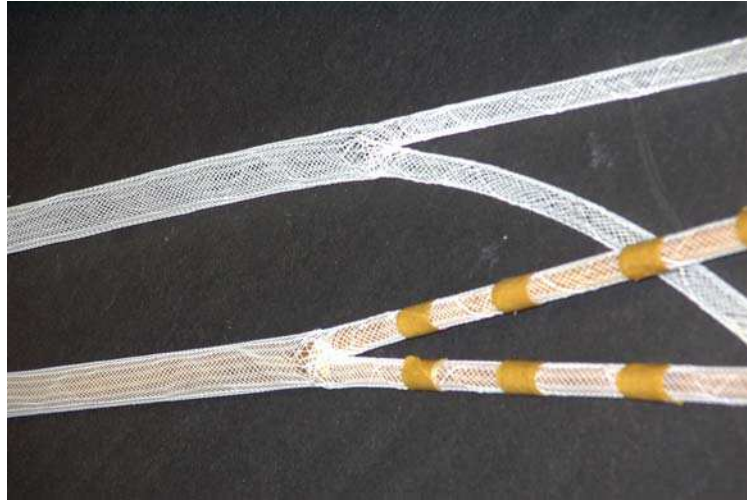
Figure 3.8: Prototype bifurcated stent (sample with tapes is method A and without tapes is method B).
