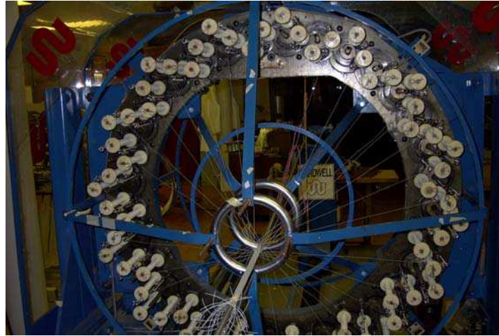
Figure 3.10: Arrangement of spools on Wardwell braiding machine showing 32 out of 64 yarns actually braiding.
