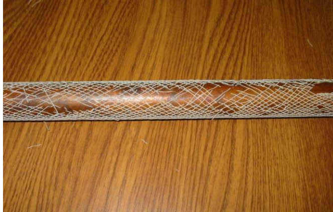
Figure 4.3: Degradation of braided sample at 226 °C (440 °F).
