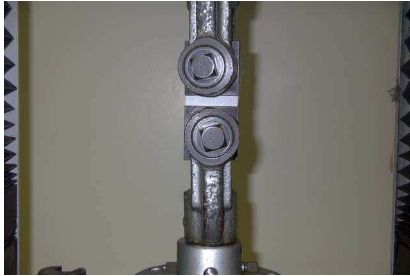
Figure 3.16: Experimental arrangement for tubular woven samples on Instron (cross-machine direction)
