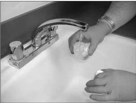
Holding the bottle under the water flow with cap in other hand
