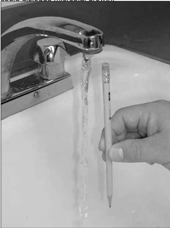
Adjusting the water to about 1/4 inch diameter flow
