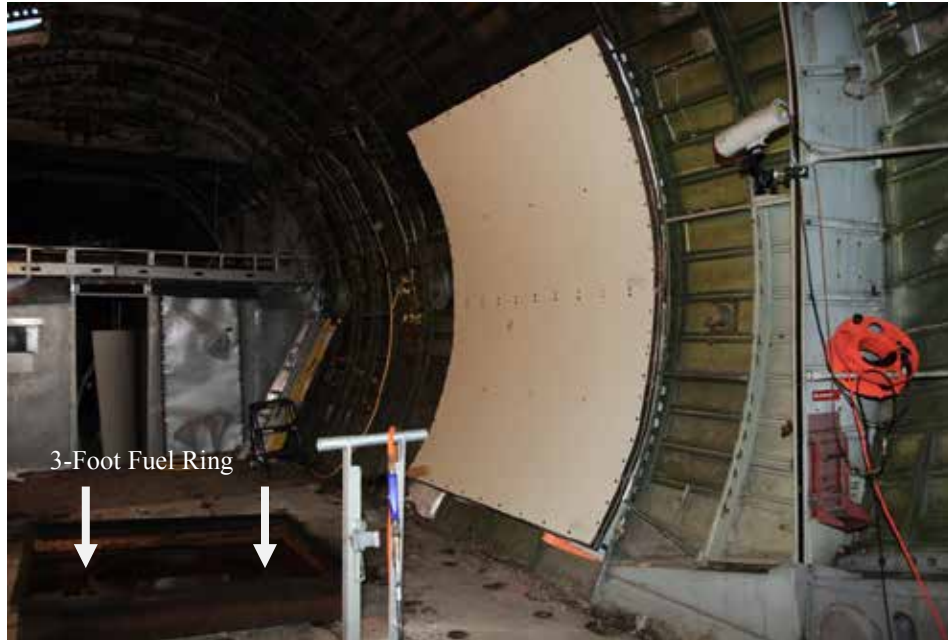
Figure 16. Full-Scale Test Section Ready for Fire Heating
