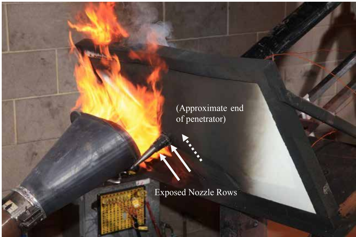
Figure 18. Incomplete Penetration During Heated Test
