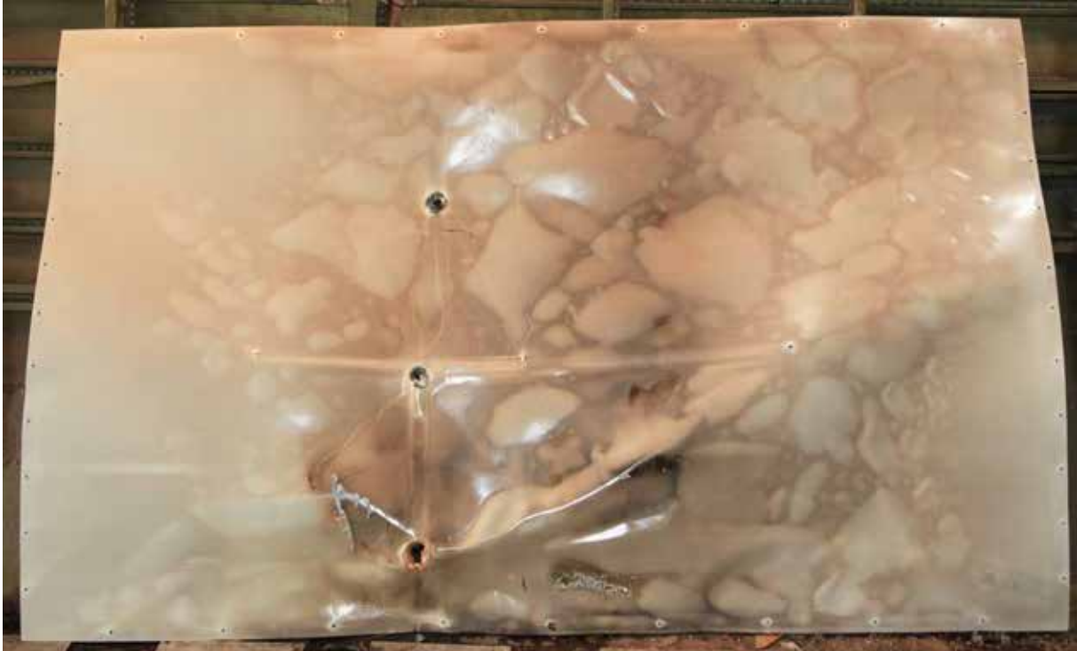
Figure 24. Posttest Backside Delamination Damage
