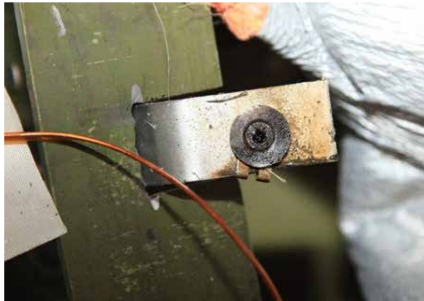
Figure 31. Screw and Washer Still Attached to Bracket
