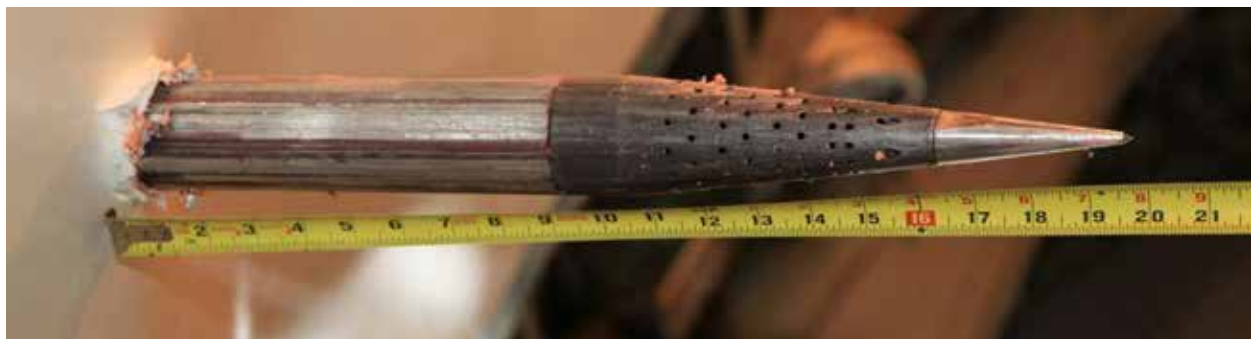
Figure 21. Complete Penetration During Ambient Test
