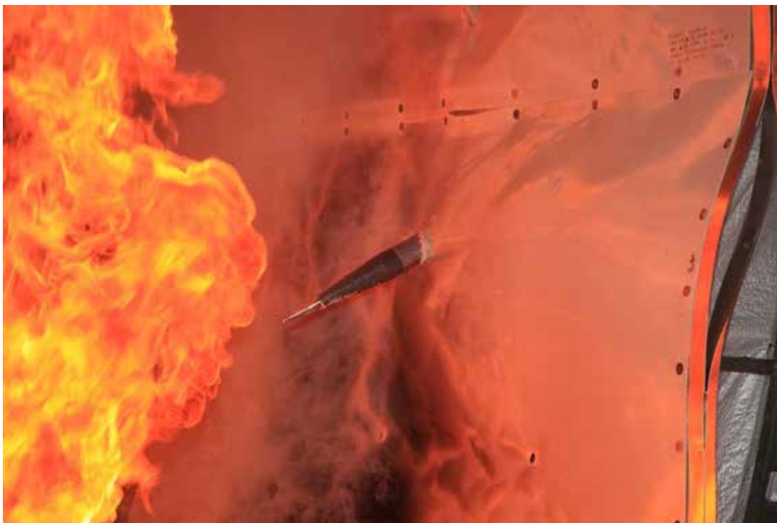
Figure 23. Complete Penetration During Full-Scale Test
