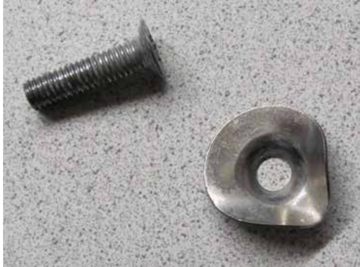
Figure 32. Washer Bent From Penetration Force
